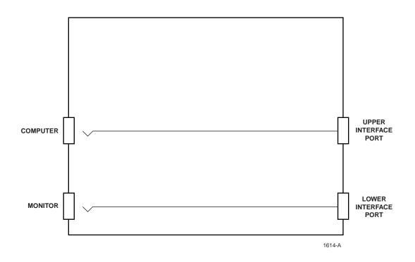
Figure 2-9. Patch Interface Simplified Circuit Diagram
